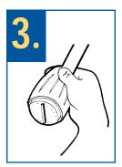
Thread the new showerhead onto the shower arm by hand. When it is hand-tight, turn on the water. Any leaks probably will indicate cross-threading or insufficient sealing tape. To stop
