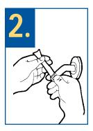
Clean the shower arm threads with steel wool. Wrap the threads with Teflon tape one and one-half times in a clockwise direction. Turn on the water to flush out any scale that may have
