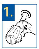
Remove your old showerhead with a wrench, pliers or vise-grips, using counter-clockwise turns. Apply a penetrating oil to dissolve any scale build-up on
